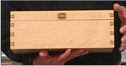
**Rick's** second box was made from **Maple**, with double dovetail joints at the corners, using contrasting **Walnut** secondary dovetails to enhance the joinery, producing a striking visual effect. Also of interest were the mortised **Brusso** lid supports:
